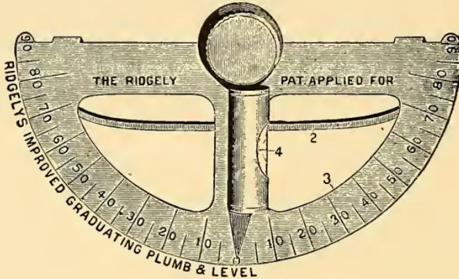
Fig. 65—Graduating Plumb and Level.
