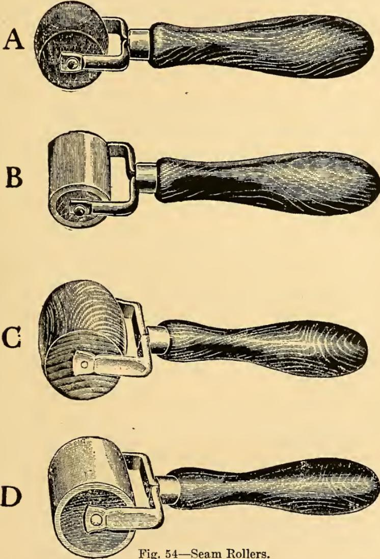
Fig. 54—Seam Rollers.
